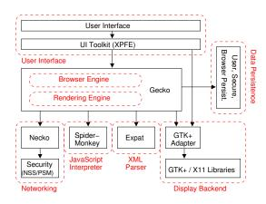
Figure 3. Architecture of Mozilla
